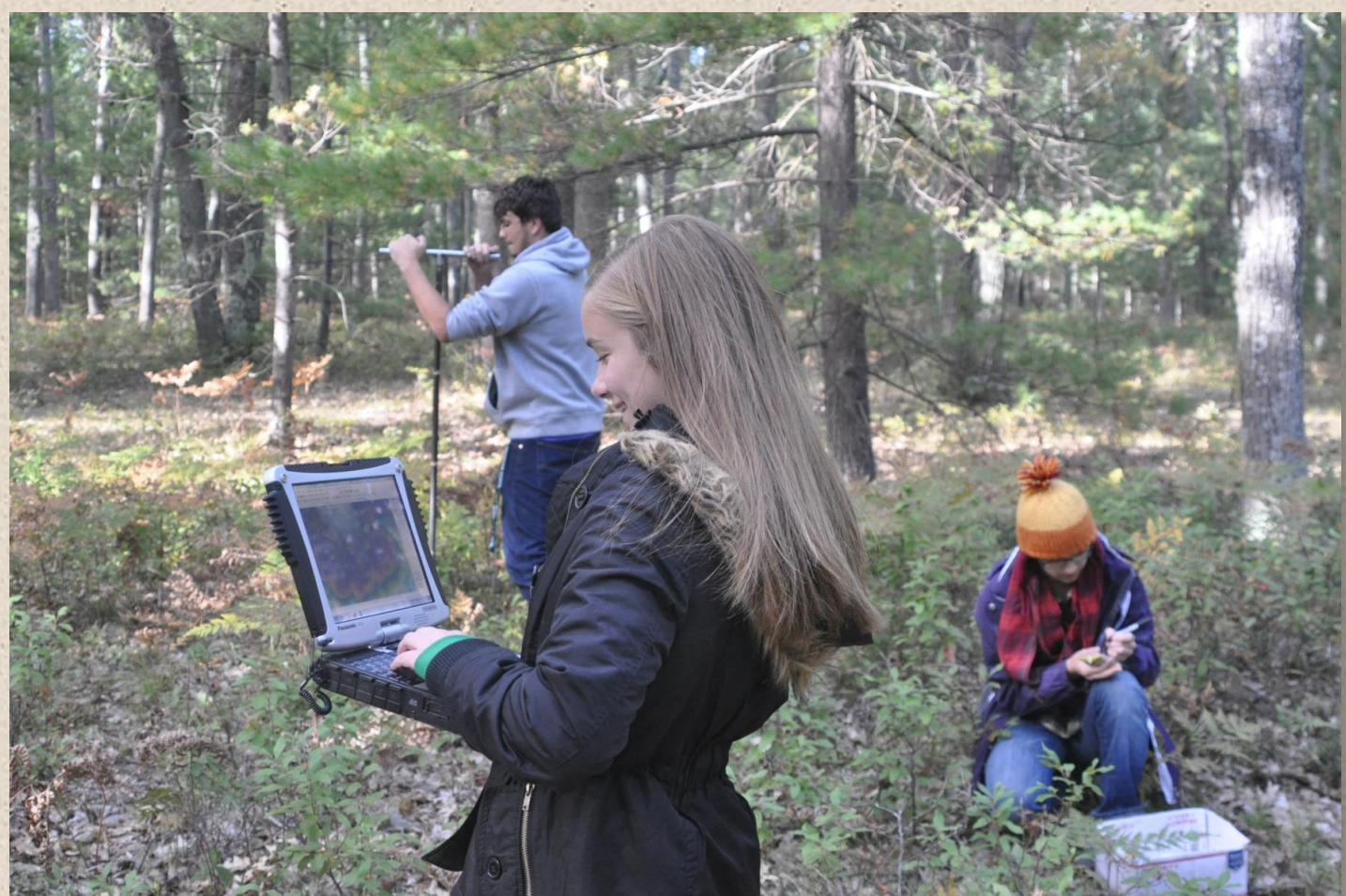
Figure 3. Fieldwork, illustrating (left) augering into the Cottage Grove Delta, while other students enter date into the ArcGIS shapefile, and mark sample bags, and (right), a completed OSL sample.
